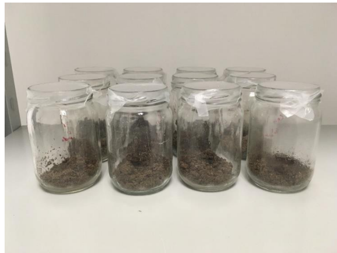
Figure 5. Glass test containers used for the F. candida reproduction test, performed based on the ISO procedure 11267.
