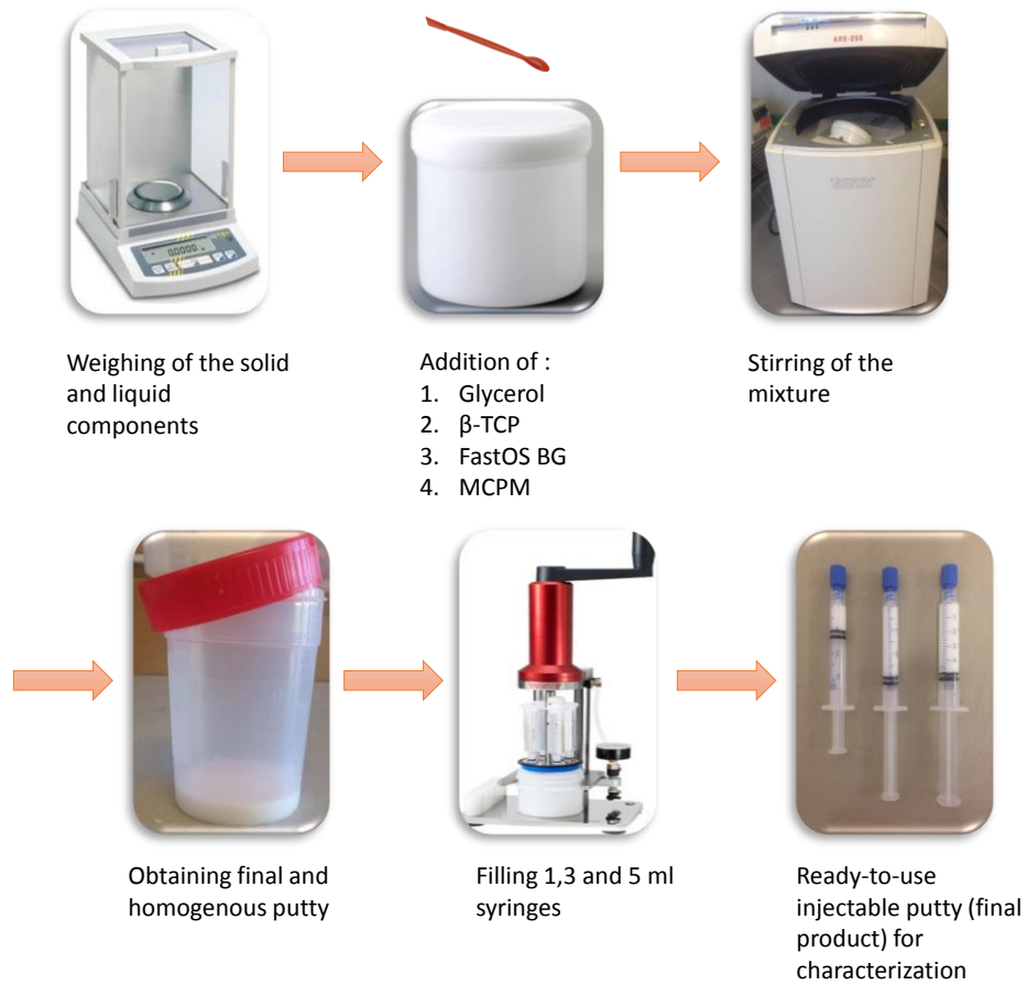
Figure 9 – Putty preparation scheme.
