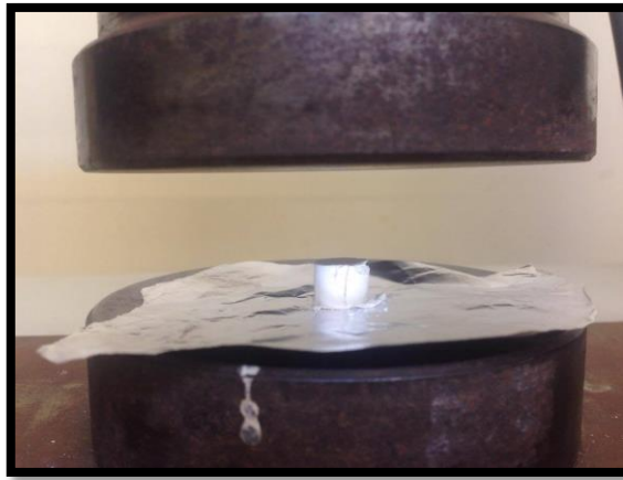
Figure 12 – Compressive strength measurement of the putty (after failure).
