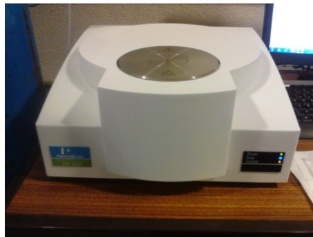
Figure 50 Differential Scanning Calorimeter (DSC) – Perkin® Elmer 4000
