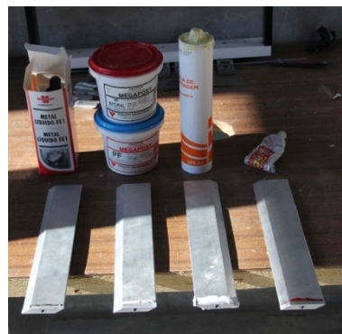
Figure 53 Some solutions to seal the PCM macrocapsules
