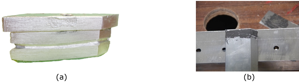
Figure 54 (a) Aluminium blade end cap; (b) Window blade with epoxy on the external surface
