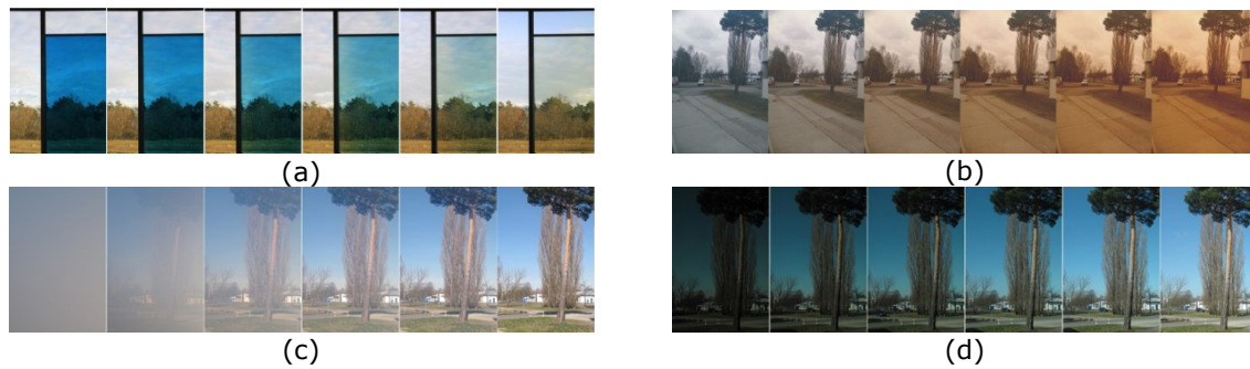
Figure 42 Switching process using (a) thermochromic, (b) electrochromic (c) electrochromic and (d) thermochromic laminated glass
