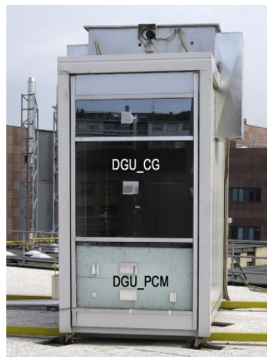
Figure 16 Experimental test cell with the two glazing systems (DGU_PCM and DGU_CG) [30]
