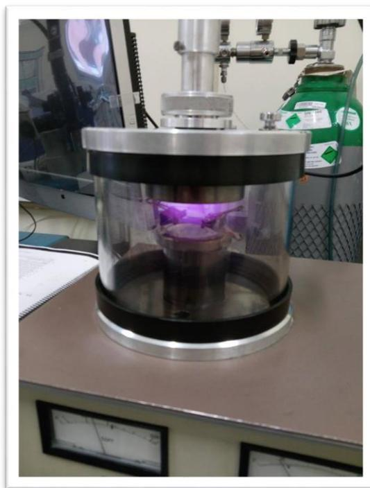
*Figura 26- Método de Sputtering utilizando o equipamento Polaron Equipment Limited SEM Coating Unit E5000.*
