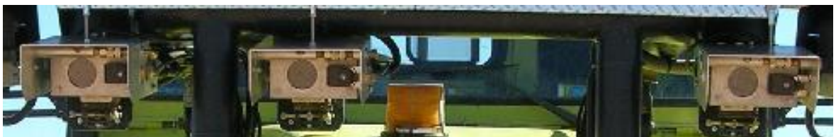
Figure 2.15: Trinocular System used in TerraMax [16].
