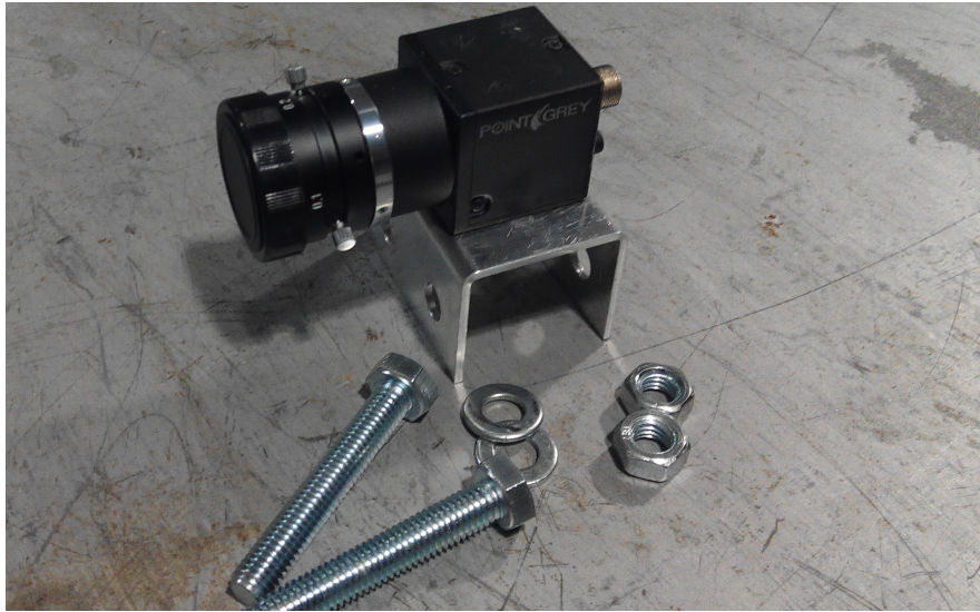
Figure 3.9: Camera skate - assemble to the rail profile.
