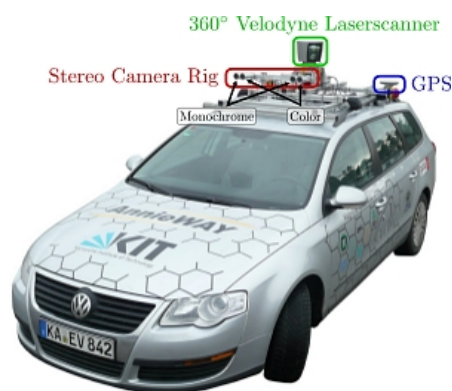
Figure 2.19: Position and description on each sensor of Annieway [18].
