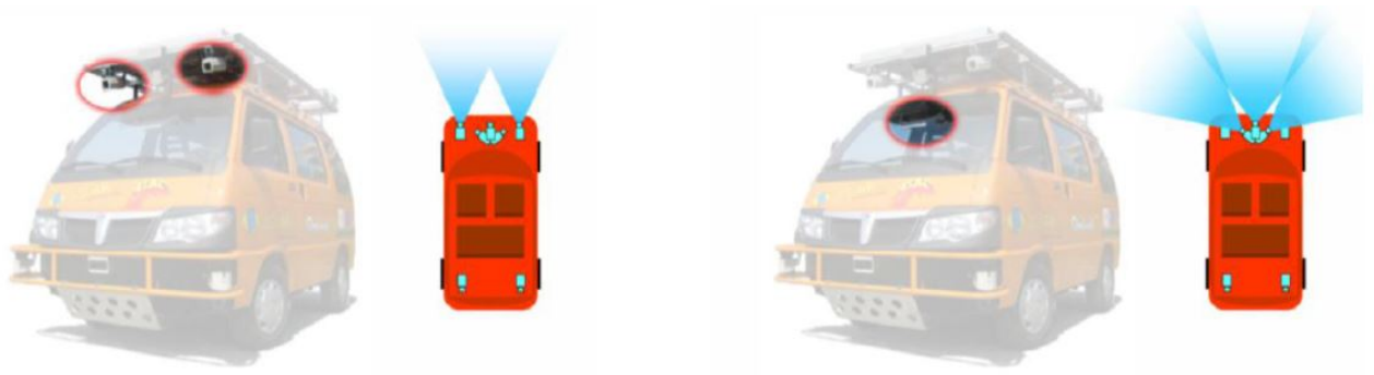
Figure 2.17: Left: frontal stereo vision systems to detect lane markings and obstacles; right: frontal panoramic vision system to locate the leader vehicle [42].
