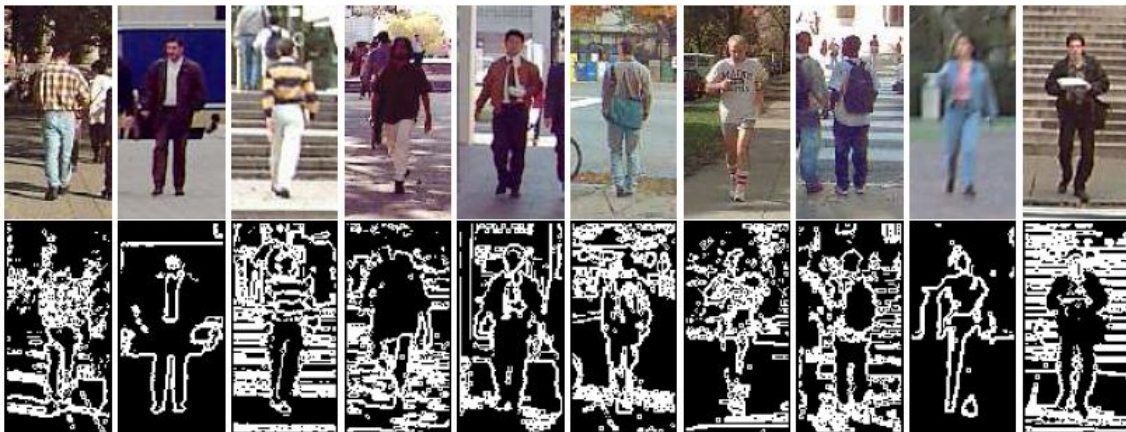
Figure 2.8: Original image and the corresponding edge maps generated by a sobel filter [27].
