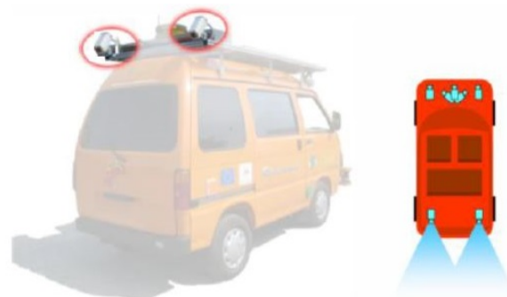
Figure 2.18: Back stereo system used to detect upcoming traffic and obstacles during backup maneuvers [42].
