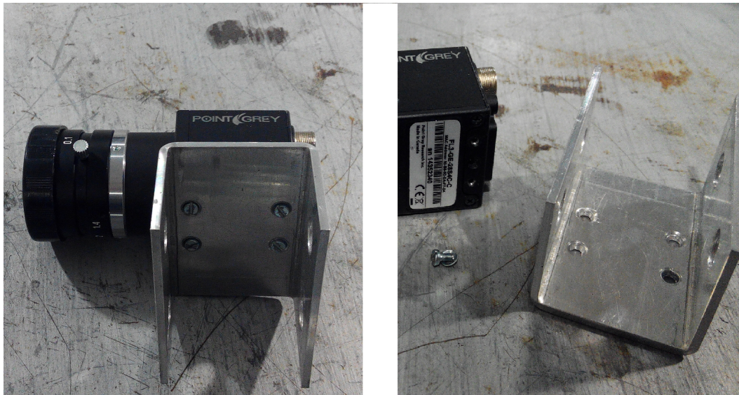
Figure 3.8: Camera skate - assembling to the camera.
