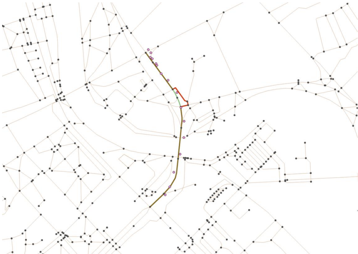
Figure 11. The test case with 75% of correct way segments found. The pink dots represent the GPS data and the green line marks the way segments that correspond to the data. The red line marks the trajectory found by the algorithm.
