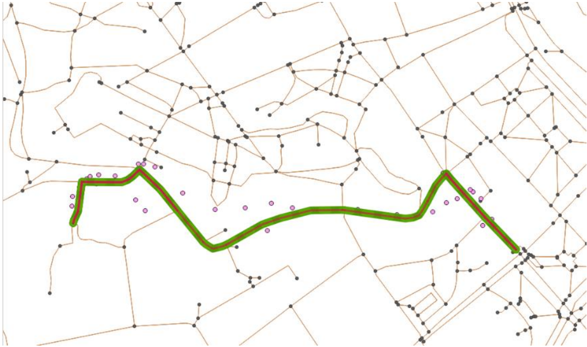
Figure 10. The test case with all correct way segments found. The pink dots represent the GPS data and the green line marks the way segments that correspond to the data. The red line marks the trajectory found by the algorithm.
