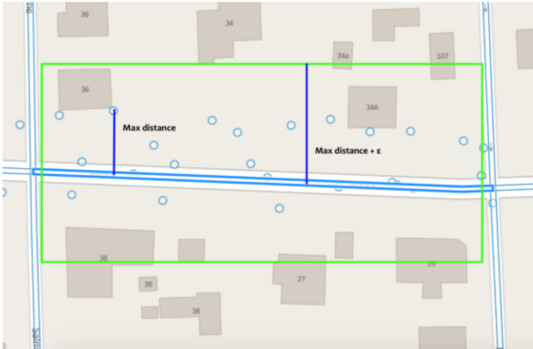
Figure 10. Dynamic grid cell generation principle
