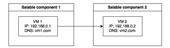
Figure 4. Connection between VMs in initial configuration
