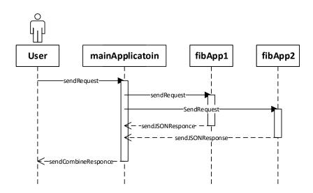
Figure 14. Sequence diagram for Parallel workflow experiment
