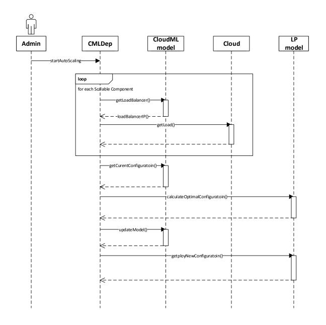
Figure 8. Auto scaling sequence diagram.
