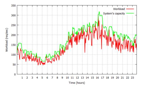
Figure 21. Workload and system capacity during parallel workflow experiment third component
