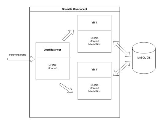
Figure 10. One component deployment configuration in case of increased workload
