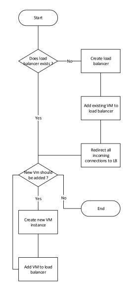
Figure 3. Scaling up algorithm
