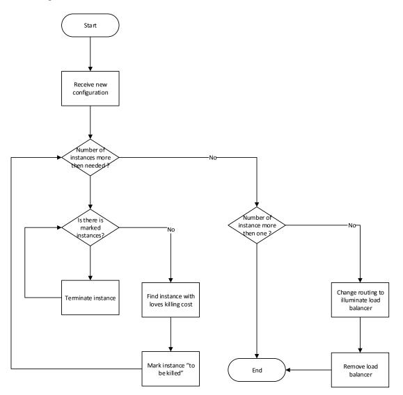
Figure 6. Scaling down algorithm
