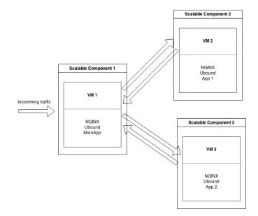
Figure 15. Initial deployment model from experiment with multiple scalable components
