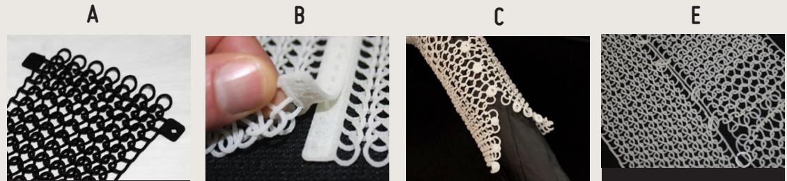
Figure 5. Different attachment-variations are modeled, (a) button that can be attached when rotated, but will not release in normal orientation, (b) push-button principle, (c) variation on push buttons, need a bit force to be attached — or released, (d) button and loop, pull or slight tension in the material will keep attachment in place, (e) different rings that can connect different knitted panels. The thin rings can be printed in nylon to have enough rigidity for the yarns not to fall out again. The thick ring is printed from TPU, and needs more mass to be stiff enough.
