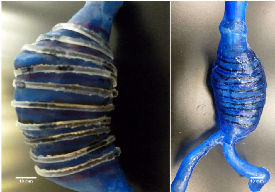
Figure 6-12 PUR fibers attached to the wax inner mold (left) and as a part of the final anisotropic AAA physical replica (right).
