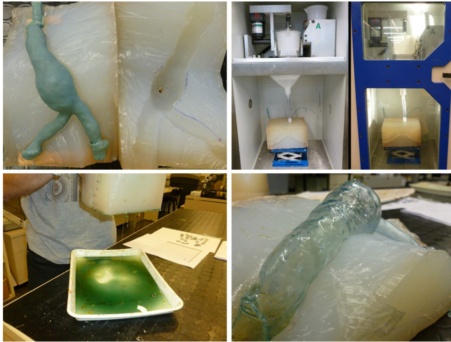
Figure 5-6 Vacuum casting process for the artery: silicone mold with the wax mold inside (top-left), mold and PUR resins ready for casting inside the MCP 4/01 vacuum casting machine (top-right), wax melting (bottom-left), and opening the mold to remove the artery (bottom-right).
