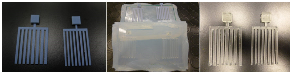
Figure 6-2 Fiber manufacturing process: AM fibers (left), silicone mold (center) and final PUR resins fibers (right).
