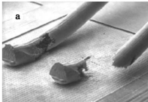
Figure 3.15. Bond-wire heel cracking IGBT [5]
