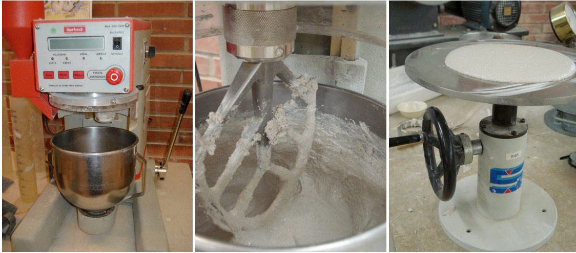
Images 3, 4 and 5. A mortar mixer, the mixing process of the mortar paste and determining the consistence of the fresh mortar, in a flow table
