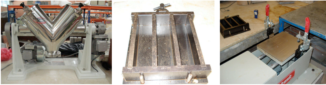
Images 4, 5 and 6. V type mixing machine, three gang mould for mortar samples (40 x 40 x 160 mm) and jolting table for compaction.
