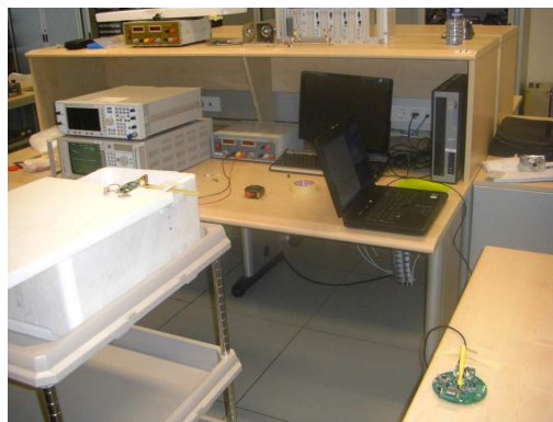
Fig. 6.41. Setup of the entire implanted smart system, with base station and control unit.
