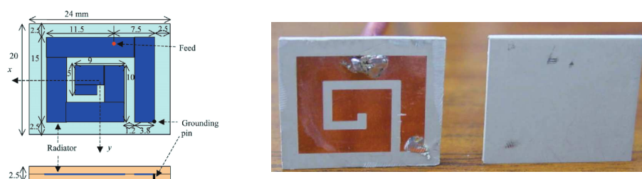
Fig. 2.29. Microstrip spiral folded antenna topology with short circuit: Layout (left) and implemented design (right) [106].
