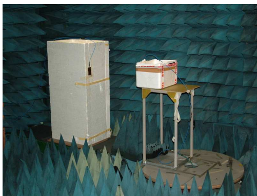
Fig. 6.26. Near field measurements setup for reader to implant communications.
