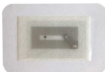
Fig. 2.26. Deployable smart diagnostic skin patch GT200 for fever monitoring [96].
