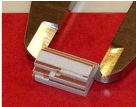
Fig. 2.31. Example of a multilayer microstrip antenna for MedRadio frequency [109].
