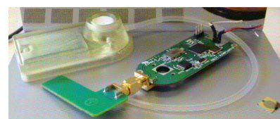
Fig. 4. The developed platform with an EBI sensor and a test antenna.
