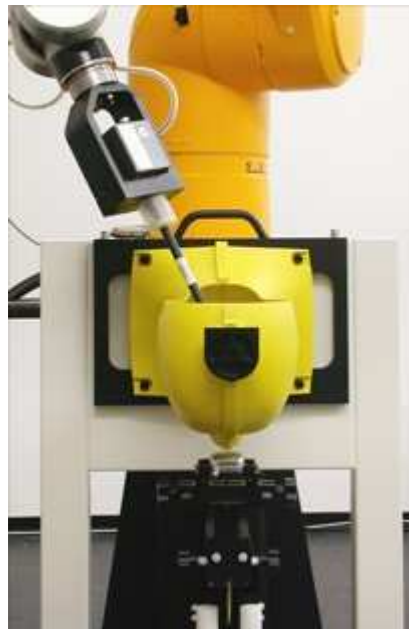
Fig. 2.19. Face down liquid phantom of the SAM v6 with robotic arm [80].
