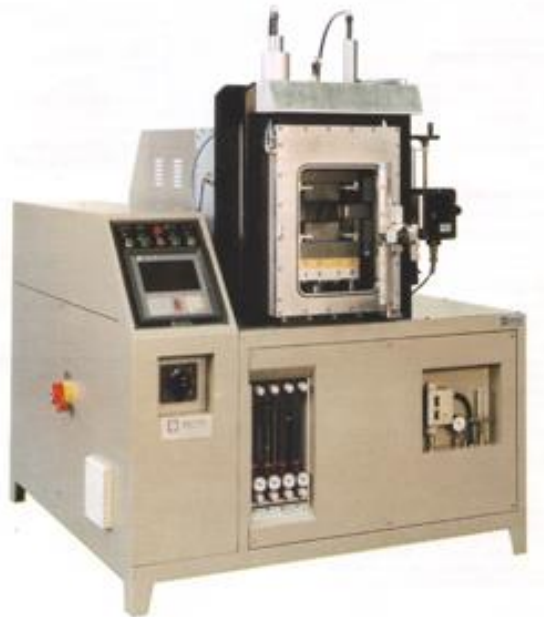
Figure 3.1: Hot- pressing machine (Sintris 10STV) employed for powder consolidation.
