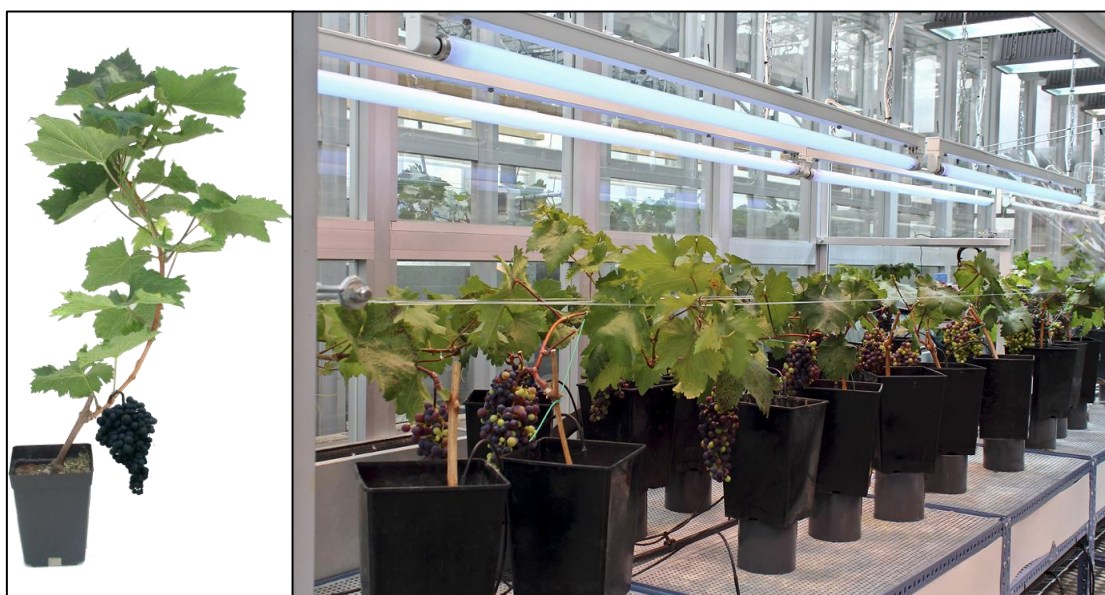
Figure 14. Fruit-bearing cutting and experimental set up inside the glasshouse with UV-B lamp array placed above the plants.
