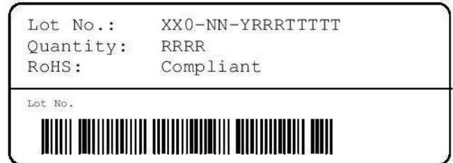
**Figure 14:** First label on reel: XX = Sensor Type (71 for SHT71), NN = Chip Version (04 for V4), Y = last digit of year, RRR = number of sensors on reel divided by 10 (200 for 2000 units), TTTT = Traceability Code.
