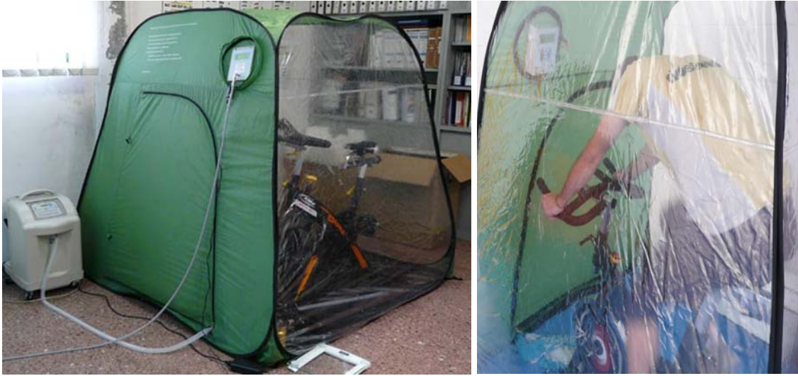
Figure 1. Normobaric-Hypoxic tent equipped for research [143] and used to trained climbers for an Everest expedition, 2011 (unpublished results).
