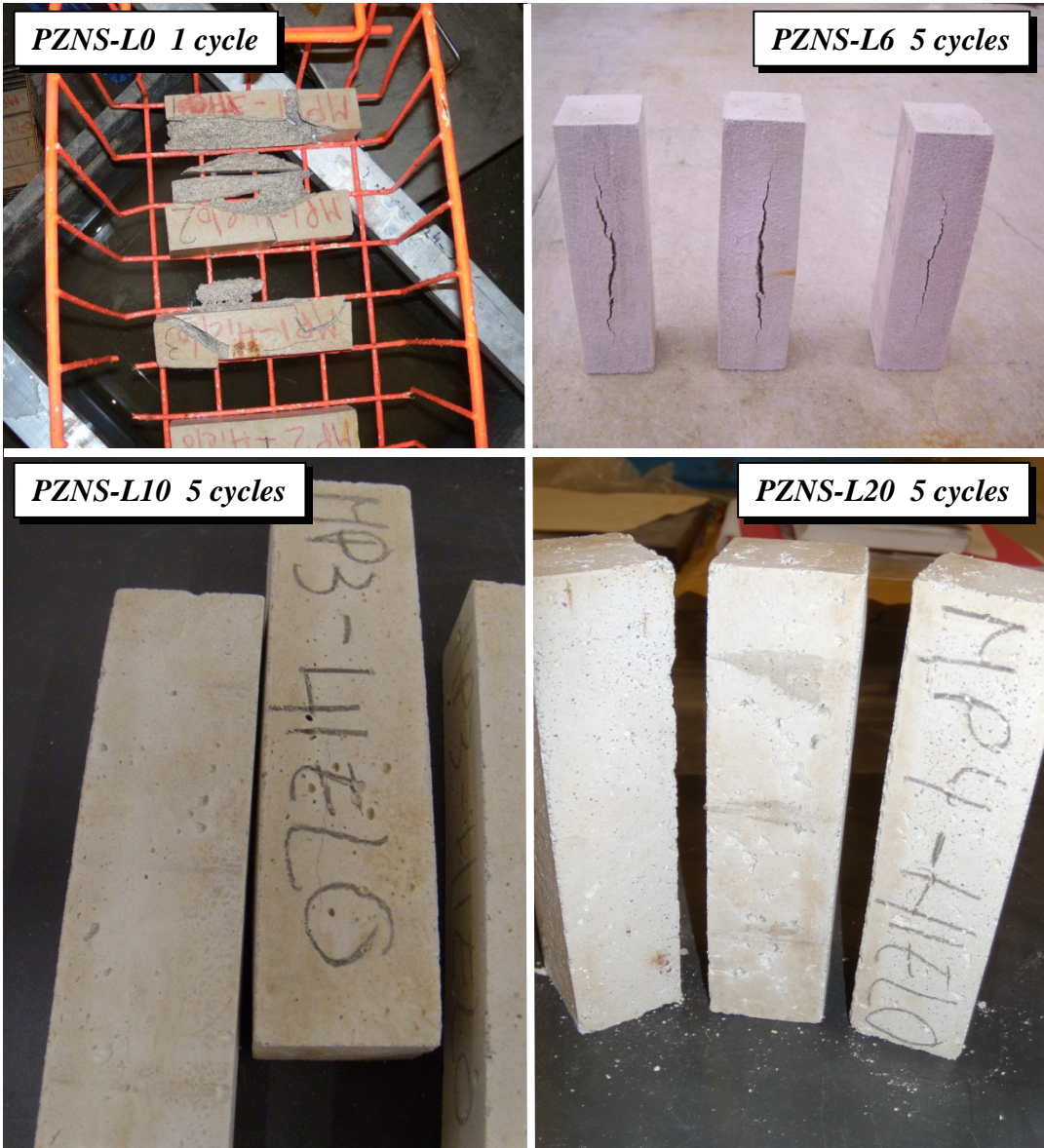
Figure 12. Samples' condition after freeze-thaw cycles: PZNS-L0, after just 1 cycle and PZNS-L6, PZNS-L10 and PZNS-L20 after 5 cycles.
