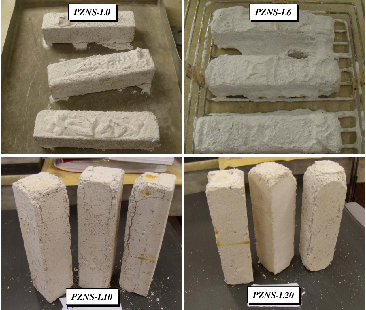
Figure 16. Damaging effect of the sulfate attack on the samples after 4 ageing cycles.
