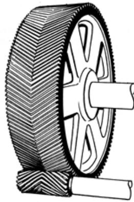
Figura 7.4: Helicoidales Herringbone.
