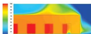
Figure 12: CFD results for the whole temperature distribution (in °C) in the end of Experiment 2
