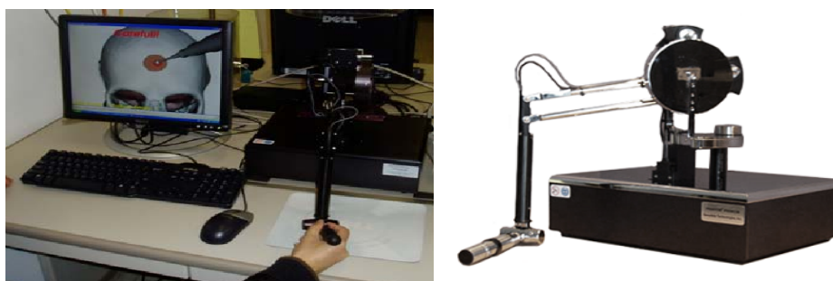
Figure 1.10: Freehand-controlled bone drilling simulator including a Sensable 6 DoF Phantom Premium device (He and Chen, 2006)
