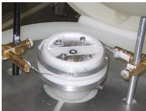
Figure 4.7: Photograph of the modified spin-coating chuck.
