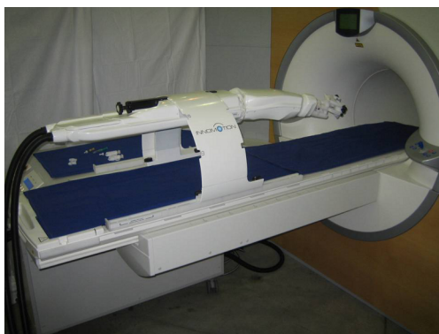
Figure 2.8: The Innomotion robot, used for CT and MR guided needle-based procedures. Copyright Innomedic GmbH. Used with permission.
