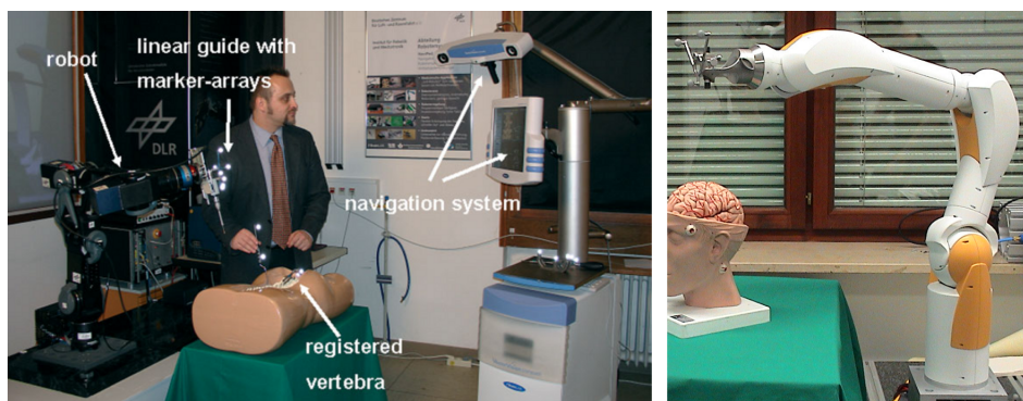
Figure 2.5: The DLR's surgical systems. Left: the prototype using the LWR II coupled with the navigation system and reflective markers. Right: the Kinemedic robot, successor of the LWR II. Left figure reproduced from (Ortmaier et al., 2006a). Copyright 2006 John Wiley and Sons Ltd. Right figure: Copyright Institute of Robotics and Mechatronics, DLR. Used with permission.
