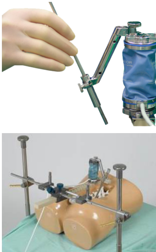
Figure 2.1: Top: the SpineAssist robot with an instrument guide. Bottom: SpineAssist mounted over the Hover-T system. Copyright Mazor Robotics Inc. Used with permission.
