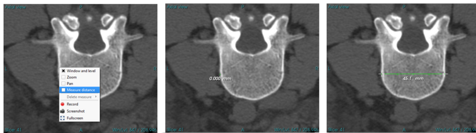
Figure 4.2: The Measure Distance tool in action: after its selection from the context menu, the user should click on two points to define a new measure.
