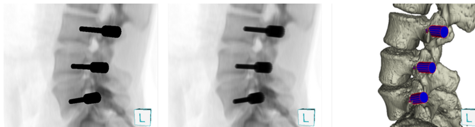
Figure 4.3: viewit-Spine's transfer styles for volume rendering: X-ray with geometric props (left), X-ray with volumetric props (centre) and Bone (right).
