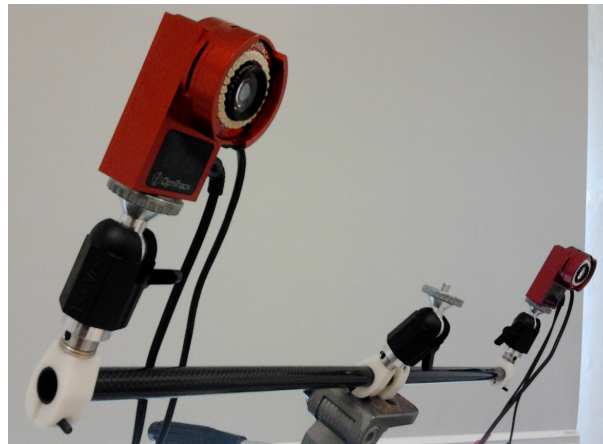
Figure 7.1: The OptiTrack motion capture system, configured with a stereo pair of V100:R2 cameras.
