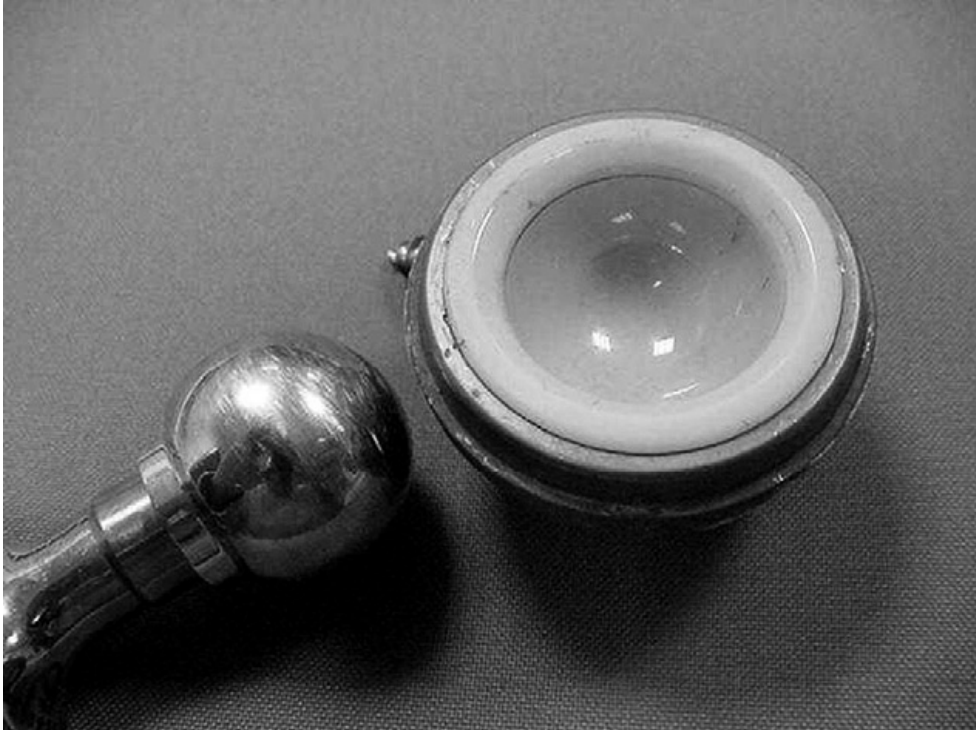
Fig. 3 Photograph of the retrieved components showing that the bearing surface was a stainless steel head and an alumina ceramic acetabular inlay. Macroscopic wear was evident on both surfaces.
