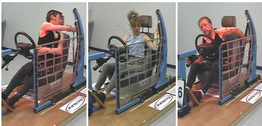
Figure 5.27: Strategies of reaching the safety belt: Right hand strategy (left), Left hand up strategy (centre) and Left hand down strategy (right). From (Dufour et al., 2003).
