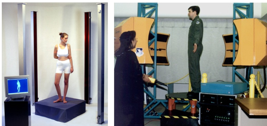
Figure 2.8: Left: Vitus Pro 3D whole body scanner. Right: Cyberware WB4 3D whole body scanner.
