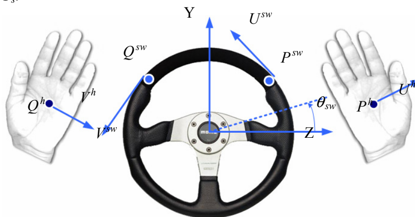
Figure 5.15: Points and vectors on the steering wheel and both hands used to define driving constraints of the model.
