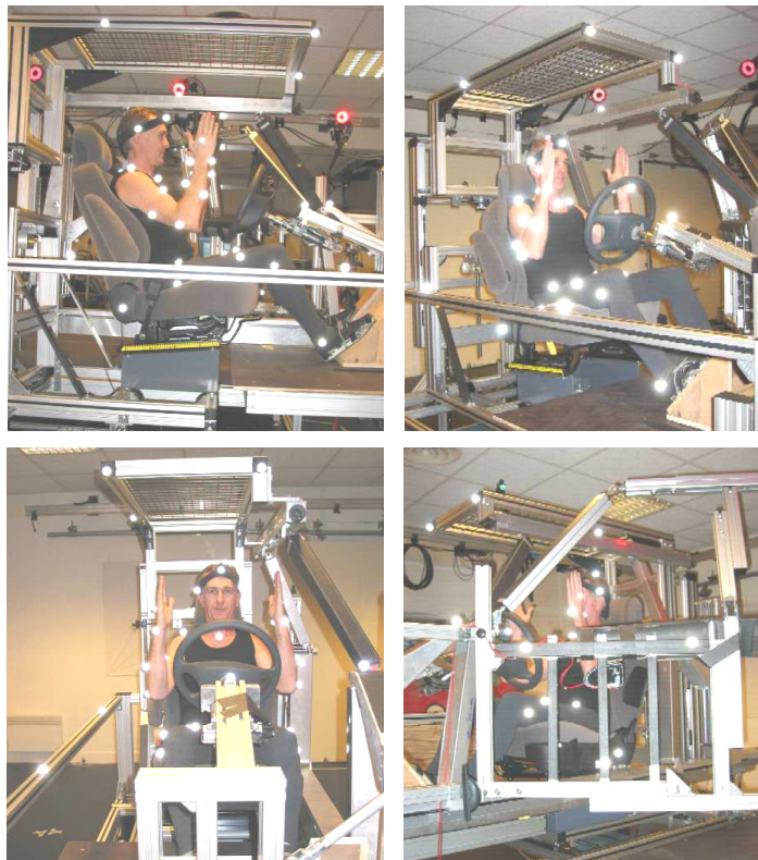
Figure 5.18: Four photos of the seated posture used for anatomical calibration with PCMAN in the door handling experiment. Reproduced from (Dufour et al., 2003).
