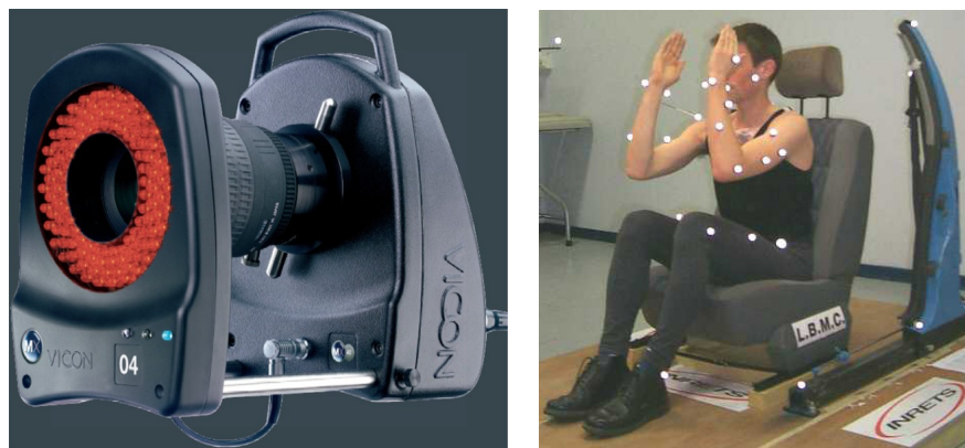
Figure 1.1: Left: Vicon MX40 motion capture camera and strobe around the objective. Right: Subject with markers (white spots) on his skin during the REALMAN project.
