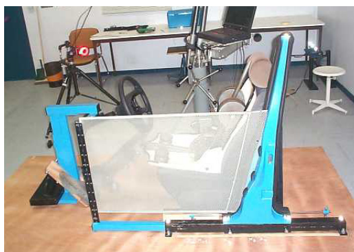
Figure 5.28: Vehicle mock-up used during the safety belt handling experiment. Reproduced from (Dufour et al., 2003).
