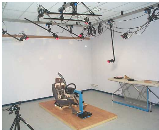
Figure 5.29: Layout of the nine cameras of the motion capture system used in the safety belt handling experiment. Reproduced from (Dufour et al., 2003).
