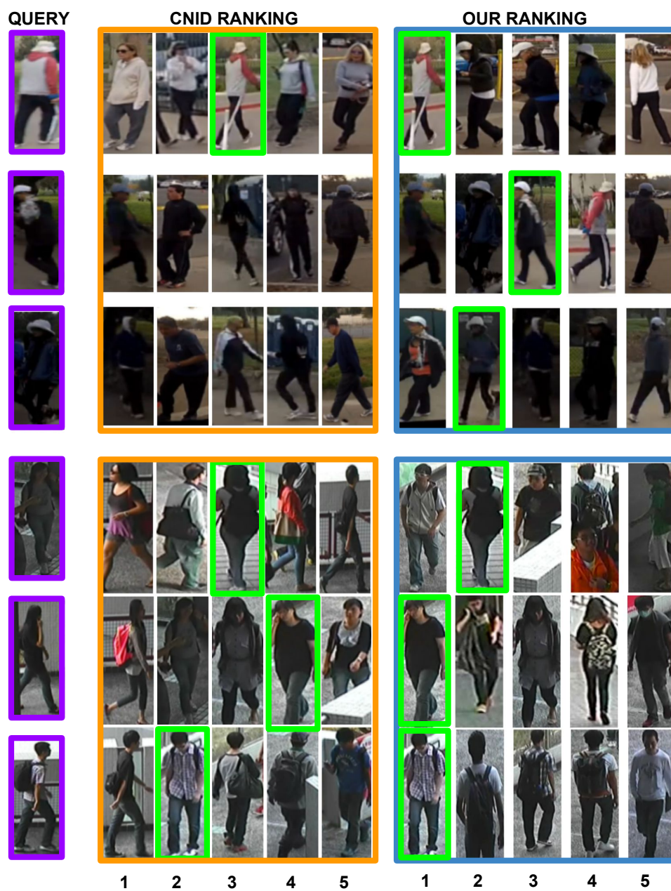
Figure 5.9: Example Ranking Results. Qualitative results, comparing the rankings produced by CIND [2] (yellow) and our method (blue). The top three rows are results from the CRP dataset. The bottom three are from CUHK03. Query images have purple borders and the correct matches in the candidate sets have green borders. For a discussion of these results see Sec 5.6
