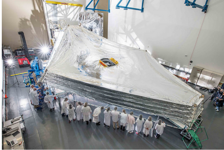
(a) Full-sized JWST sunshield post deployment test. Credit: Northrop Grumman (NASA, 2015).
