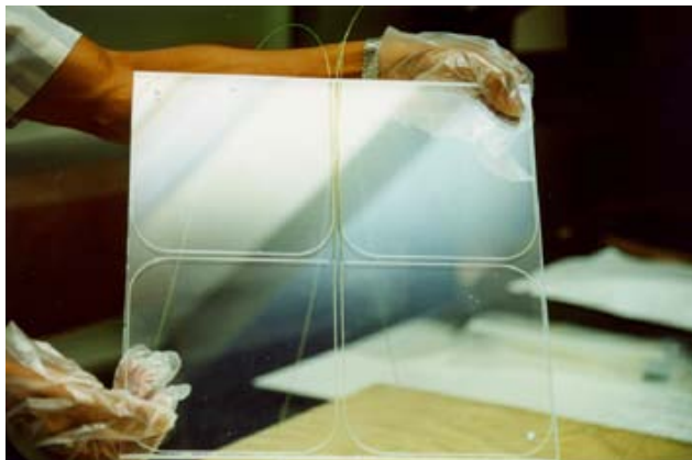
Figure 5.28: A photograph of a HO scintillating tile with the embedded WLS.
