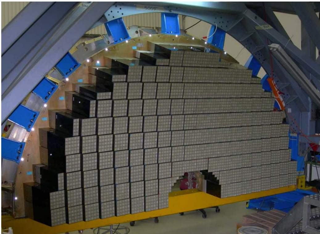
Figure 5.15: A photograph of a EE Dee instrumented with crystals.
