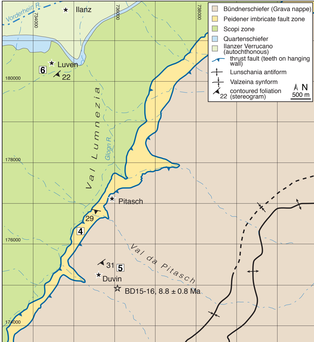
Fig. 2.14 Simplified tectonic map of Val Lumnezia and the Peidener imbricate fault zone. Foliations are taken from the stereograms shown in Figs. 2.19, 2.21, and 2.22. Geology modified after Wyss and Isler, 2011, which maps out the trace of the Lunschania antiform but not the full trace of the Valzeina synform, which is estimated here with a dashed line.
