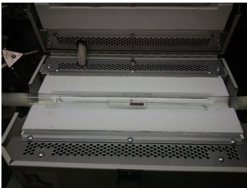
Figure 2.15. Custom chemical vapor deposition (CVD) system for the growth of \text{MX}_2 polycrystalline thin films.
