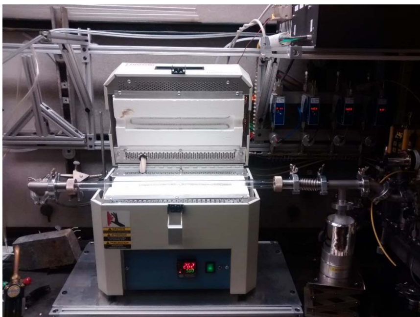
Figure 2.15. Custom chemical vapor deposition (CVD) system for the growth of \text{MX}_2 polycrystalline thin films.
