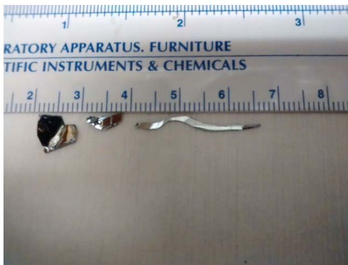
Figure 2.10. Camera image of synthetic single crystal \text{MoSe}_2 grown by chemical vapor transport method.
