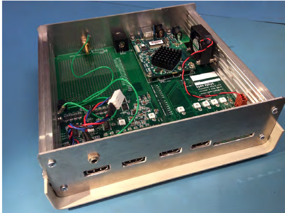
Figure 4.10: Open Ephys USB interface for using Intan RHD-class digital multiplexer headstages. This design uses an FPGA to interface the Intan digital multiplexer chips via USB. A BNC connection at the rear was programmed in software to synchronise a pulse signal from the NI PXI-6259 DAQ used to acquire data from the lock-in amplifiers. All construction was done in-house.
