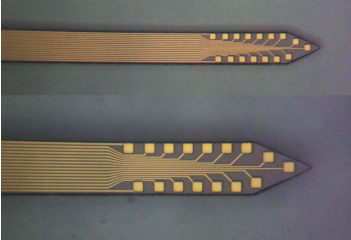
Figure 3.7: Microelectrode populated shaft tip of completed 16-channel neural probe. Note the extremely clean fabrication. The spacing between the \sim 1.25 \mu\text{m} traces at the distal end is \sim 500 \text{ nm} , which is an excellent result for photolithography. Following the fabrication steps as described, results like these are readily obtained.
