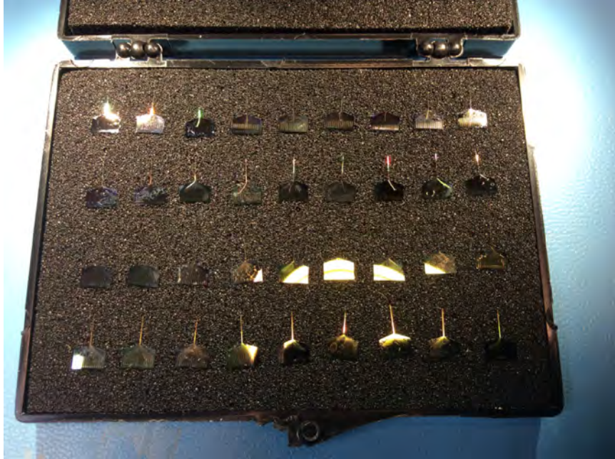
Figure 3.6: Neural probe substrates in antistatic storage case. The antistatic case prevents the extremely light probes from spontaneously becoming airborne and adhering to extraneous objects and surfaces, by dissipating static charge.
