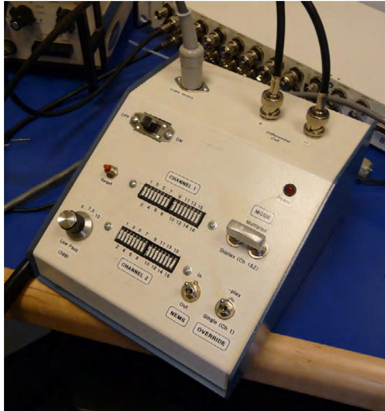
Figure 2.24: Extracellular amplifier. The amplifier was custom built to facilitate experiments with the NEMS devices, and attention was paid to proper shielding. Based on the Intan RH1016 amplifier, recording channels of interest from the neural probe could be selectively switched into each of the two independent NEMS resonators used in our multiplexing experiments.
