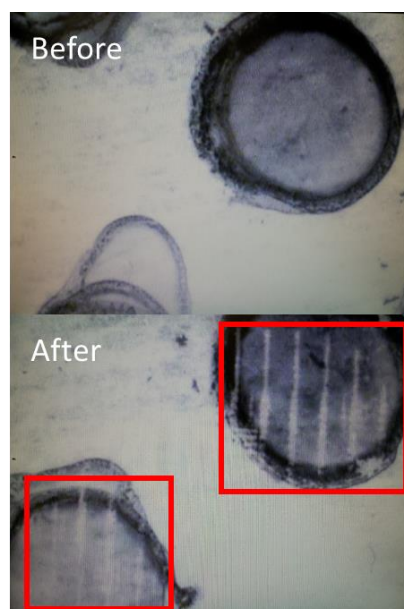
Figure 4-16 Optical image of the GNP on the MALDI slide before and after the mass deposition. The dark areas correspond to areas with GNP. A darker coloration means a higher concentration of GNP. After the deposition, lines of lighter coloration (within the red boxes) appear. These are areas where the UV laser desorbed the GNP.
