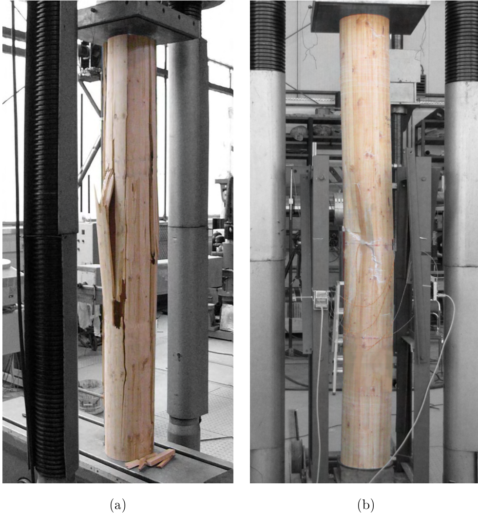
Fig. 5. Failure modes: (a) splitting of REF tube, (b) local buckling of CR85 tube and a slenderness ratio of 27 were tested in a 6MN hydraulic press. The dimensions of the specimen including the orientation of the fibre reinforcement and the test set-up of a 2.5m column are shown in Figure 4.
