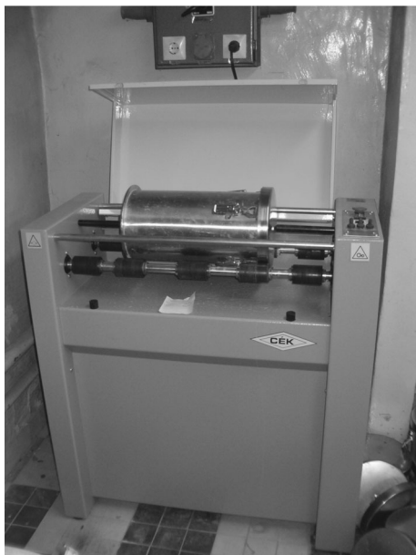
Fig. 7 Micro-Deval test equipment
