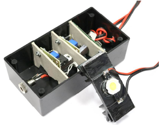
Fig. 6: The photo of the pattern generator, LED drivers (in plastic enclosure), and the power LED.
