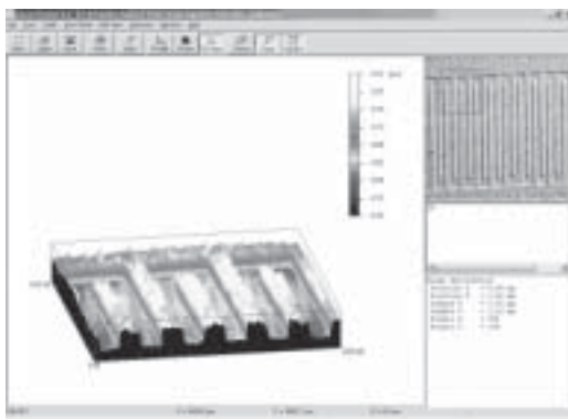
Figure 1a. Sensor on glass. Measured area in top view (Objective 20 x, Stitching 3 x 3). Height measurements for the selected profile.
