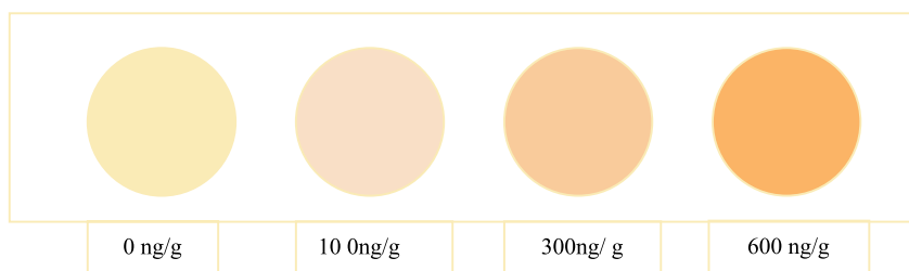
Figure 3. Similar colours to those developed in the detecting papers, using standard solutions equivalent to 0, 100, 300 and 600 ng/g
