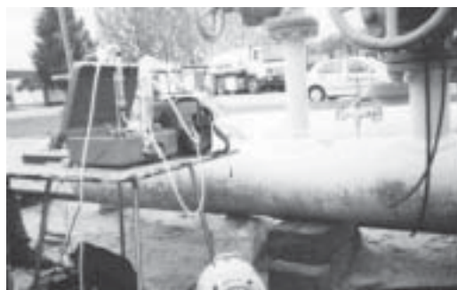
Figure 2. Mercury determination in a natural gas flow using RA-915+
