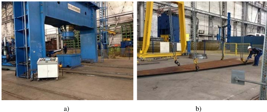
Fig. 3. a) Hydraulic press with the force of 16 MN and b) the blank, (OJSC 'Uralhimmash')
