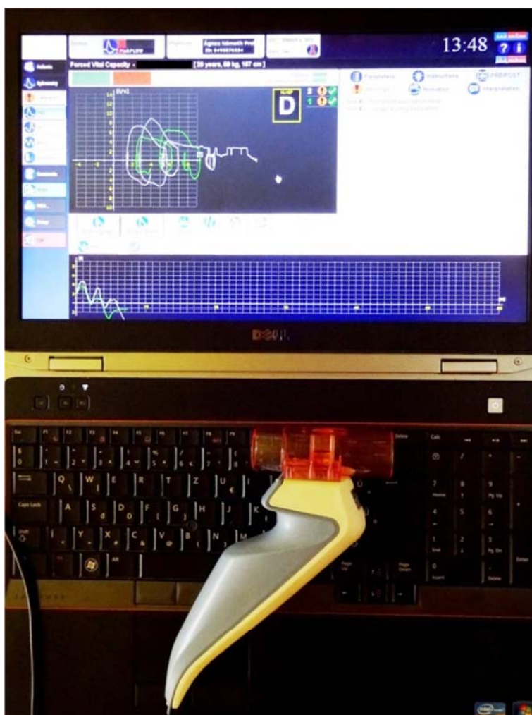
Fig. 2. Data-exchange over OTI-Hub with spirometer PDD-301/shm
