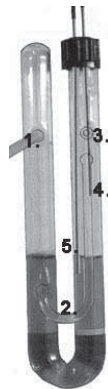
Fig. 1. Structure of the U-tube used to measure the amount of produced gas as part of the online fermentation monitoring system. Legend: 1. Gas introductory tube (from reactor); 2. transfer tube between the two legs; 3. gas outlet; 4. shorter electrode (+4.4 V voltage); 5. longer electrode (0 V voltage)
