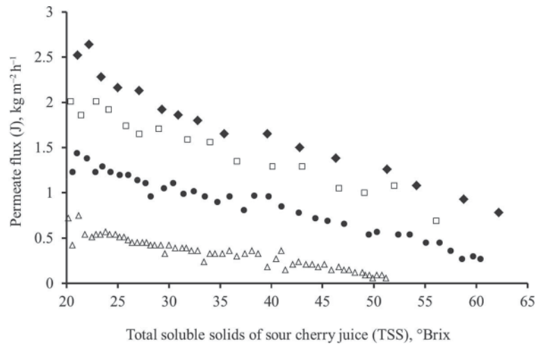
Fig. 2. Permeate flux during the concentration of sour cherry juice using different kind of osmotic agents (□: CaCl 2 ; ♦: CH 3 COOK; Δ: K 2 CO 3 ; ●: NH 4 NO 3 )
