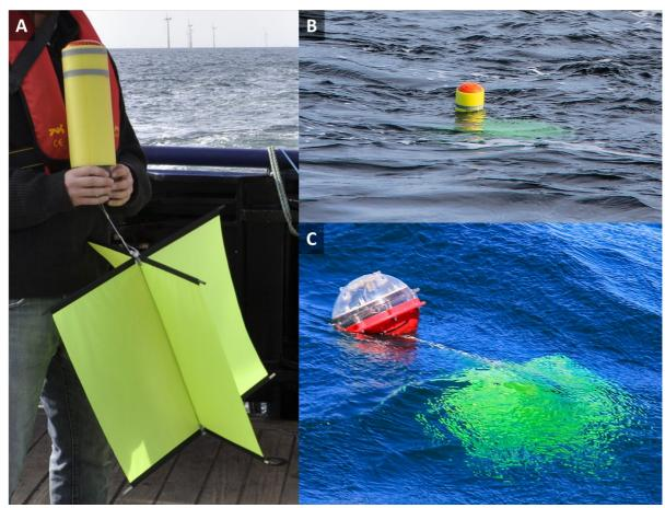
Figure 1: Drifters used during the experiment. The drifter sails were mounted 0.5 m under the sea surface and had a length and diameter of 0.5 m (A). Two kind of drifters were utilized the yellow cylinder shaped one (MDO3i) with only approx. 0.08 m above the water surface (B) and the ball shaped drifter (ODi) with approx. 0.1 m above the water surface (C). Both drifters were photographed shortly after launch and therefore the sail has not settled yet.
