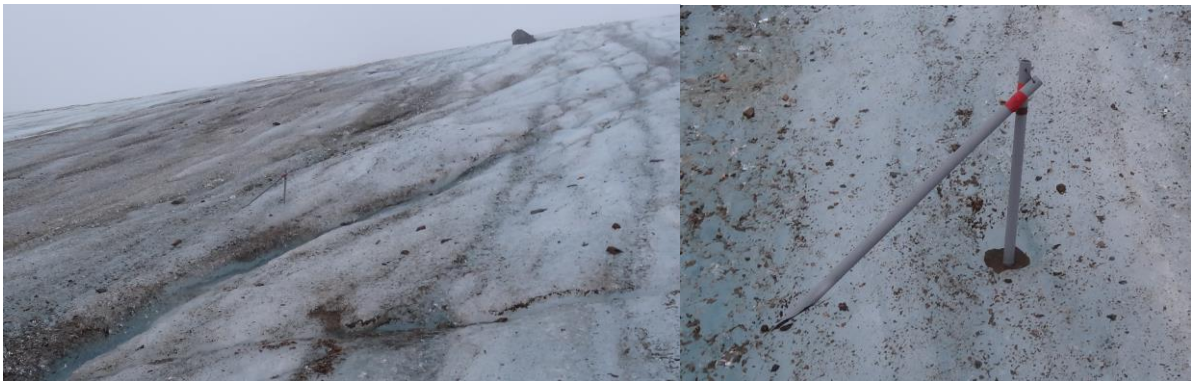
Ablation stake 2a. 17cm firn ablation, 90cm ice ablation maek -912mm w.e. (Fotos: J. Abermann)
