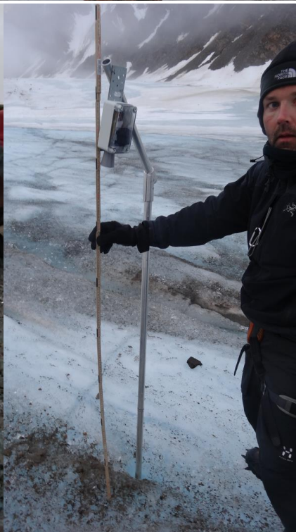
Automatic ablation sensor near stake 3 and stake 3 with 93cm ice ablation in 2017.
