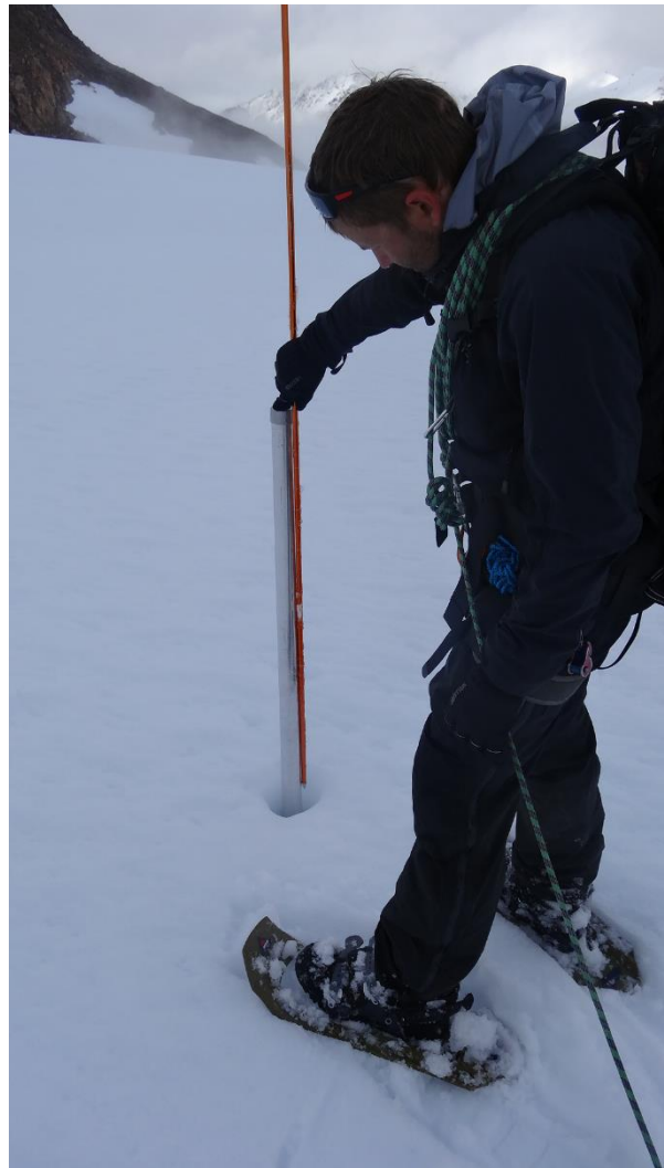
Top and bottom left: The broken AWS after being buried in 1m accumulation 2014 and 2.8m winter snow 2014/15. Sensors, datalogger and batteries have been retrieved. Right: the mast of the old AWS at stake 13, which is drilled into the ice. (Fotos: J. Abermann)
