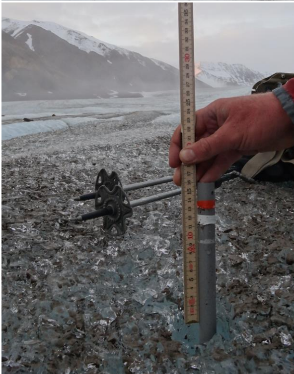
Automatic ablation sensor near stake 3 and stake 3 with 93cm ice ablation in 2017.
