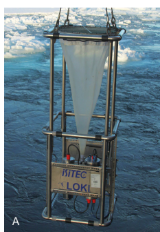
Fig. 1A: LOKI, deployed in the Fram Strait
