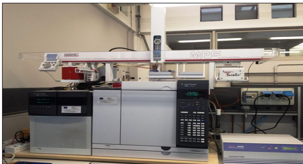
Figure 4 Agilent Technologies 7890 B GC System e Agilent Technologies 7000 C GC/MS/MS Triple Quad
