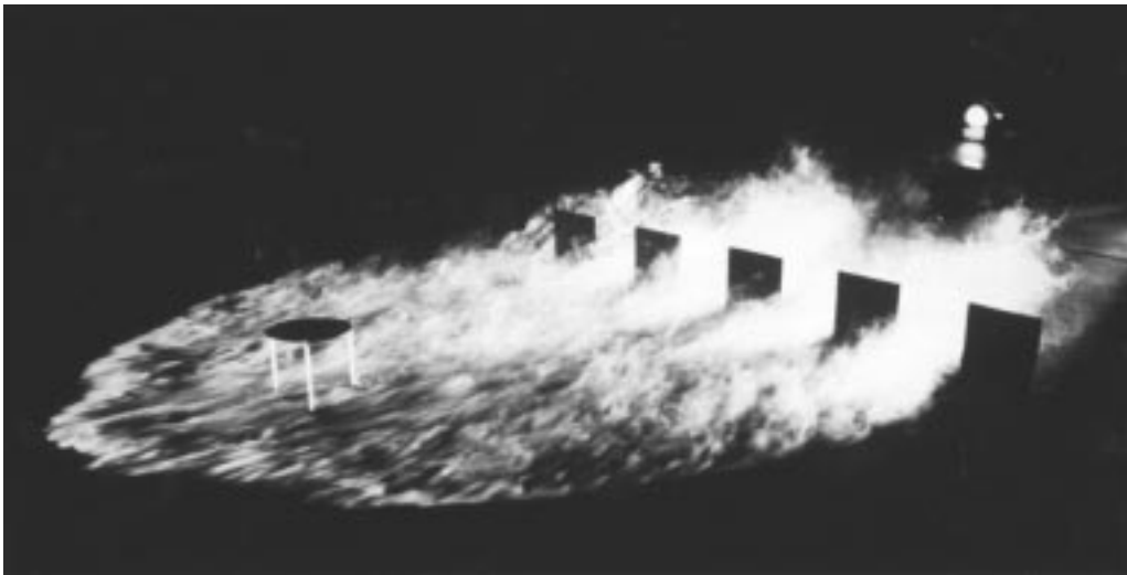
Fig. 3. - A typical view of dispersion soon after release in the presence of a crenellated fence ( Ri = 10 , H = 15.3 cm). See text for further details.
