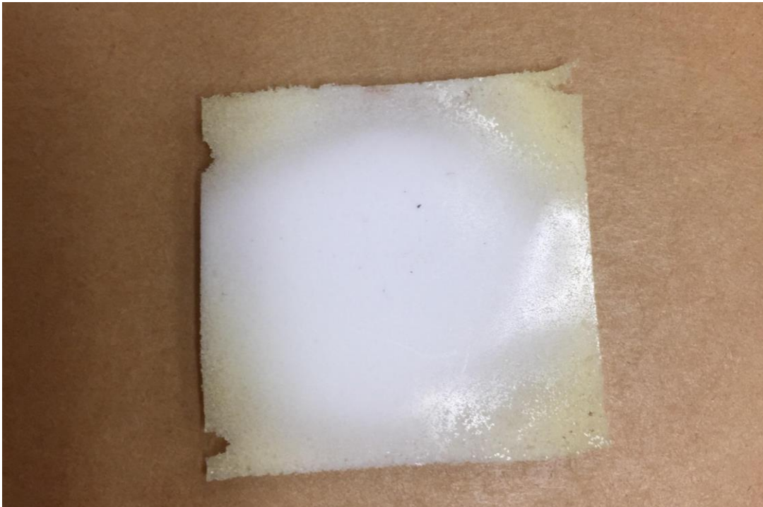
Figure 5.4 Conventional compression molding operation for disc-shaped sample of molten GUR 2122
