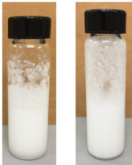
Figure 3.2 (a) GUR 2122 and glycol, 5 min after shaking. (b) Micropoly 250S and glycol, 5 min after shaking.
