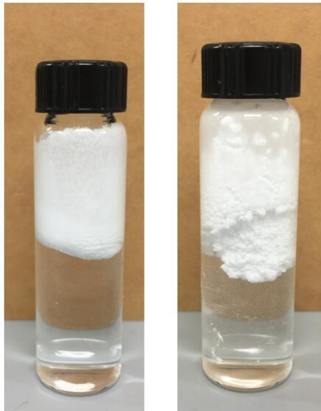
Figure 3.1 (a) GUR 2122 and water, 1 min after shaking. (b) Micropoly 250S and water. 1 min after shaking.
