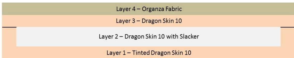
Figure 46. Layering of silicone and fabric, forming a new neck skin that allows the cricoid and thyroid cartilage to be palpated on the mannequin's neck (© 2015, Andrew L. Hosmer)
