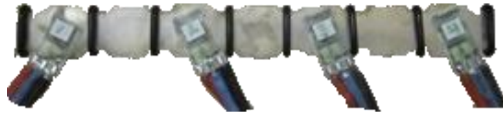
Figure 34. New mounting apparatus for the Hall-effect sensors (© 2015, Douglas A. Nelson Jr.)
