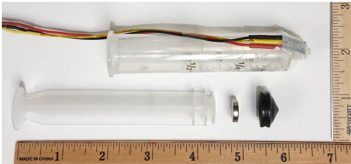
Figure 36. Modified syringe with Hall-effect sensor mounted near the tip for measuring plunger position, originally developed by Samosky (© 2016, Douglas A. Nelson Jr.)
