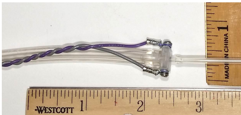
Figure 37. New conductivity sensor with wires connected to the stainless-steel electrodes (© 2016, Douglas A. Nelson Jr.)
