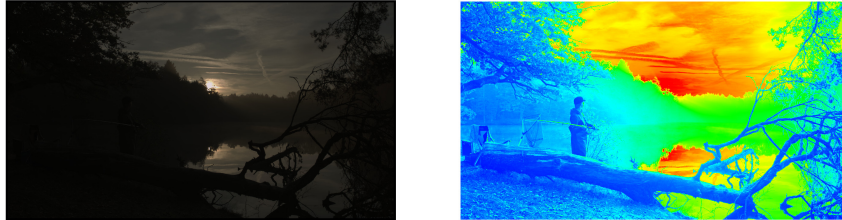
Figure 1.2: Linear representation of an HDR image (left), false color image of the HDR image (right).
