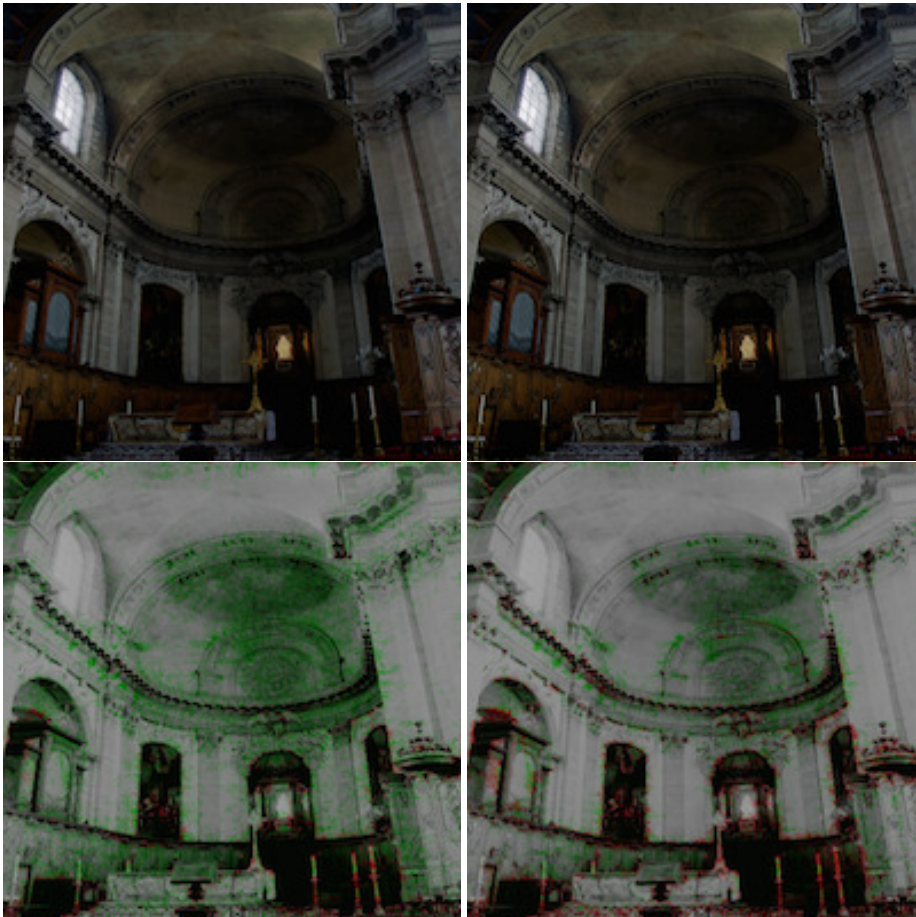
Figure 5.1: Evaluation of preprocessing stage for [Ferradans et al., 2011] TMO. Top row: input tone mapped image, output of preprocessing stage. bottom row: distortion map of the input and preprocessed image.
