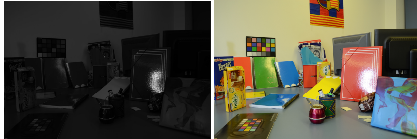
Figure 3.4: RAW sensor image (left) and final camera output (right).
