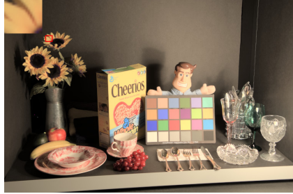
Figure 4.9: Result of color correction by [Mantiuk et al., 2009] in tone mapping (Eq. 4.12). The image has hue shifts (see the zoomed-in cropped region). Here s is computed by Eq. 4.13. Original HDR image from [Fairchild, 2007].
