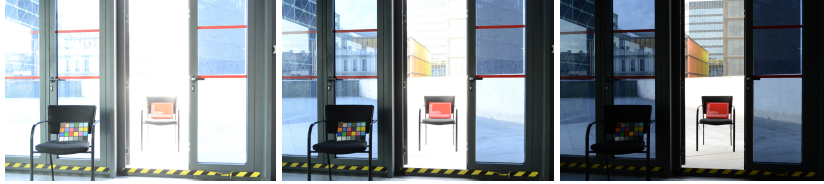
Figure 3.7: Camera output with decreasing exposure time from left to right.
