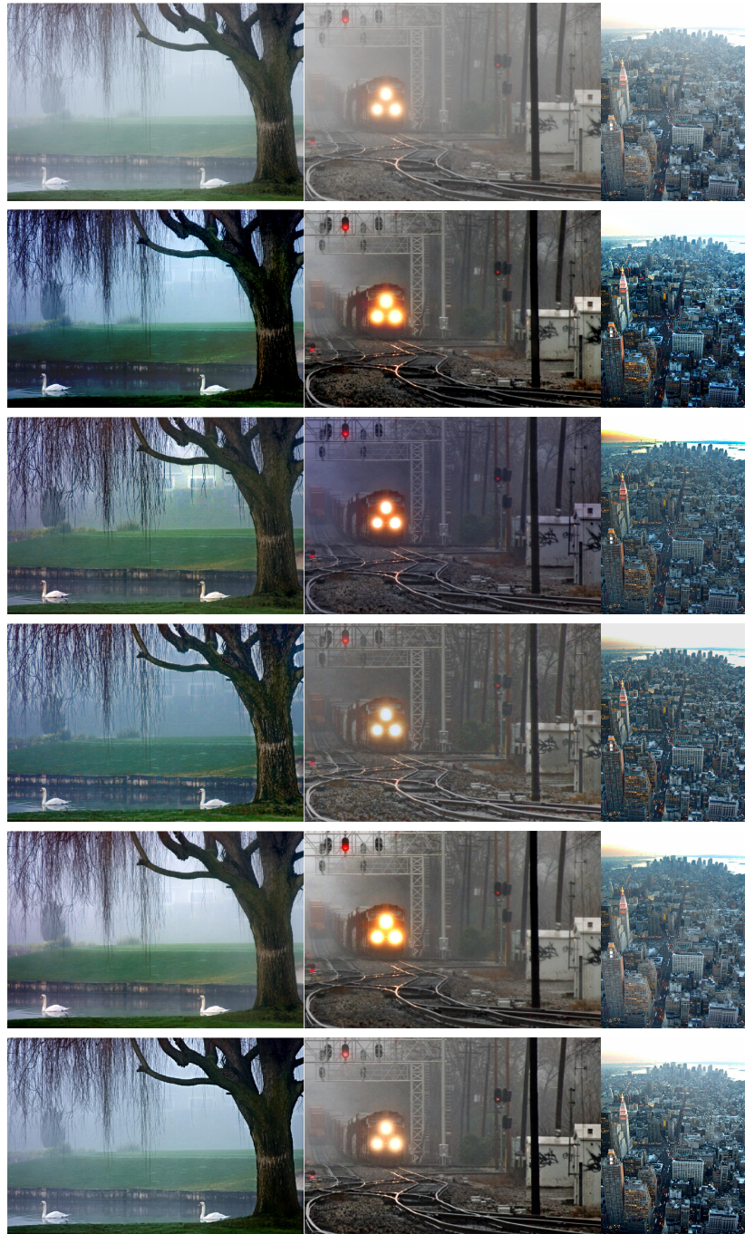
Figure 8.7: Dehazing applied to standard images. From top to bottom: Original, [Choi et al., 2015], [Meng et al., 2013], [Tarel and Hautiere, 2009], [He et al., 2011] and result of the method we propose in [Vazquez-Corral et al., 2016].
