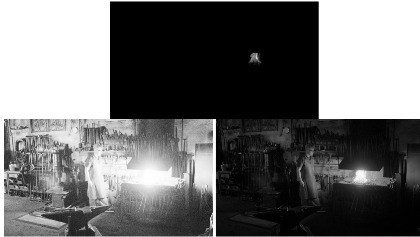
Figure 6.3: Comparison of complete histogram equalization and constrained histogram equalization. Top row: linearly scaled HDR image. Bottom row: result of complete histogram equalization of the HDR image and result of constrained histogram equalization (first stage of Algorithm 1) applied on the HDR image.
