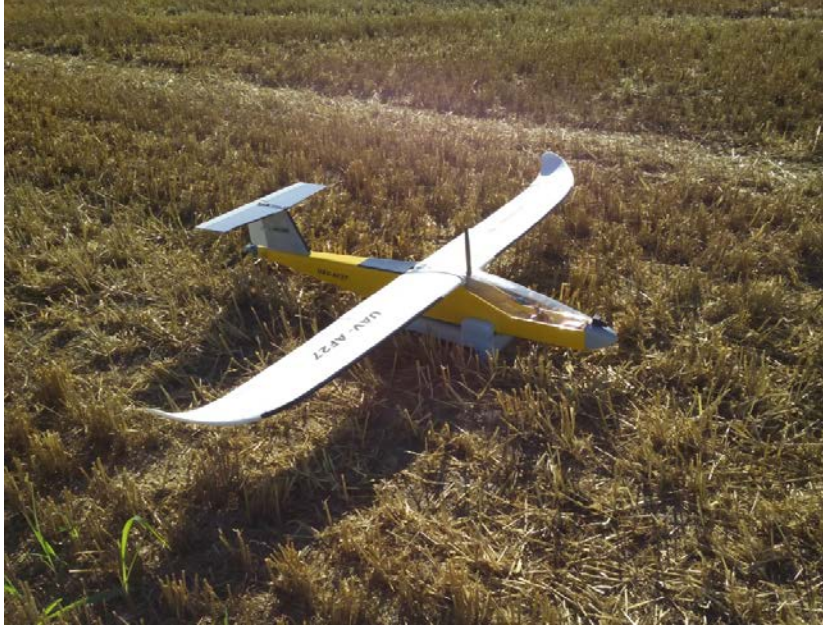
Figure 2. The Atmos-6 UAV operated by CATUAV (Moià, Catalonia, Spain), which was used as the platform for multispectral data acquisition.
