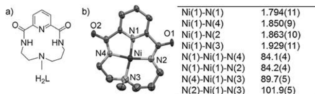
Figure 1. a) Schematic representation of H_2L . b) X-ray structure and selected bond lengths [Å] and angles [°] of 1 \cdot NaCF_3SO_3 . Hydrogen atoms and cocrystallized NaCF_3SO_3 have been omitted for clarity.
